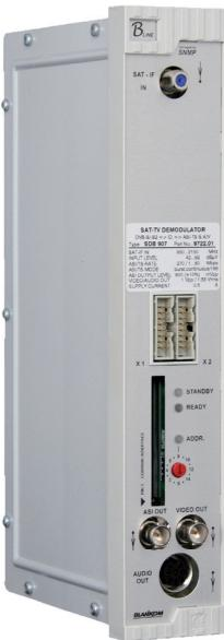
The new **SDB 907** is a modular type Satellite Receiver/Decoder. The unit receives one 8PSK/QPSK Satellite Transponder and enables demodulation into ASI-TS and decoding into one analog Audio/Video signal. The unit is equipped with a Common-Interface slot for decryption of encrypted services (Single or Multi-Service-Decryption).
